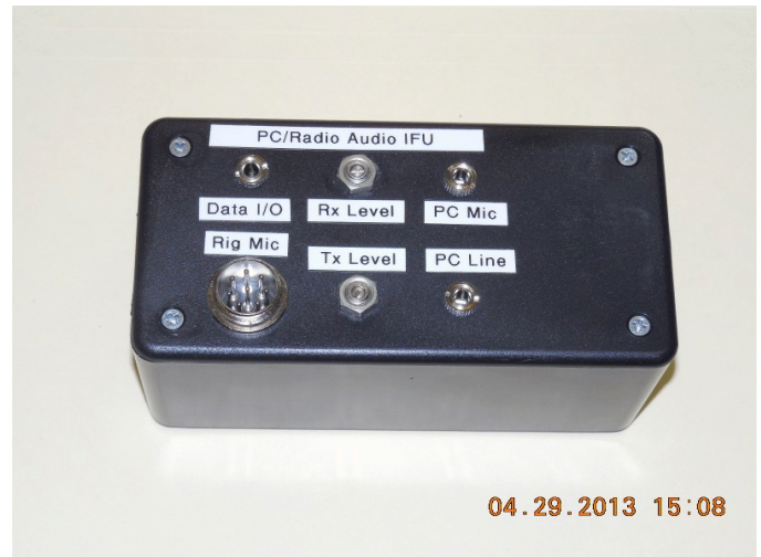
Fig. 1. The PC/Radio Interface Unit provides DC isolation and amplitude adjustment for the audio signals between the transceiver and the PC.
