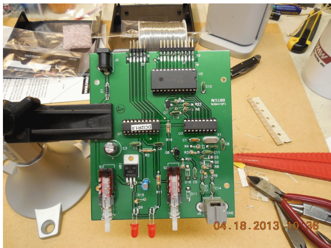
Fig. 4. The DTMF Controller decodes the DTMF tones from the telephone line and provides 16 independent logic-level outputs. This was assembled from a kit from Ramsey Electronics.
