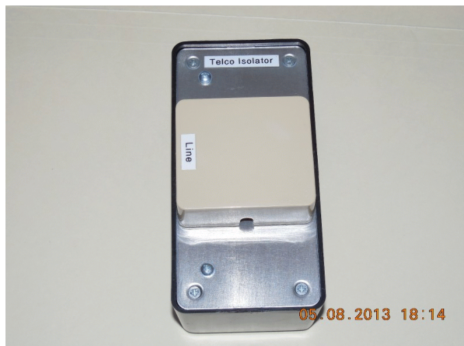
Fig. 7. The Telco Isolator is simply a 1:1 audio isolation transformer connected to the telephone line through a 2 uF non-polar capacitor.
